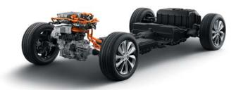
The Clarity Electric offers customers an electric vehicle that received an EPA driving range rating of 89 miles using a 161-horsepower electric motor that draws its power from a 25.5 kilowatt hour (kWh) lithium-ion battery pack. Total recharge time is just over three hours at 240 volts, and with available DC fast charging the Clarity Electric can achieve an 80-percent charge in as little as 30 minutes. It carries an EPA fuel economy rating of 126/103/114 MPGe (city/highway/combined).
