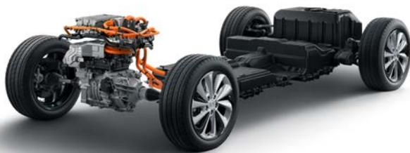
The Clarity Electric offers customers an electric vehicle that received an EPA driving range rating of 89 miles using a 161-horsepower electric motor that draws its power from a 25.5 kilowatt hour (kWh) lithium-ion battery pack. Total recharge time is just over three hours at 240 volts, and with available DC fast charging the Clarity Electric can achieve an 80-percent charge in as little as 30 minutes. It carries an EPA fuel economy rating of 126/103/114 MPGe (city/highway/combined).
